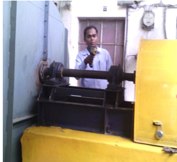
Bearing Temperature Measurement
