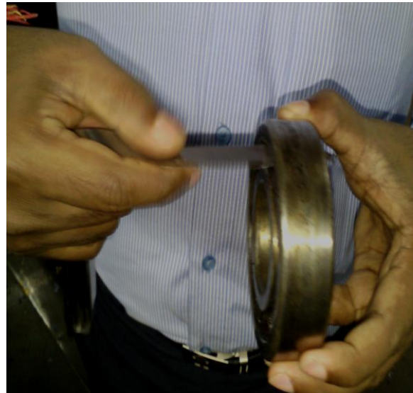
Bearing clearance Measurement
