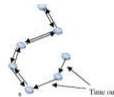
Figure 6 AODV: forward path formation
